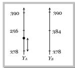
Probable frequency of A is 390 Hz and 378 Hz and After loading the beats are decreasing from 6 to 4 so the original frequency of A will be  $n_2 = n_1 - x = 378$  Hz.
